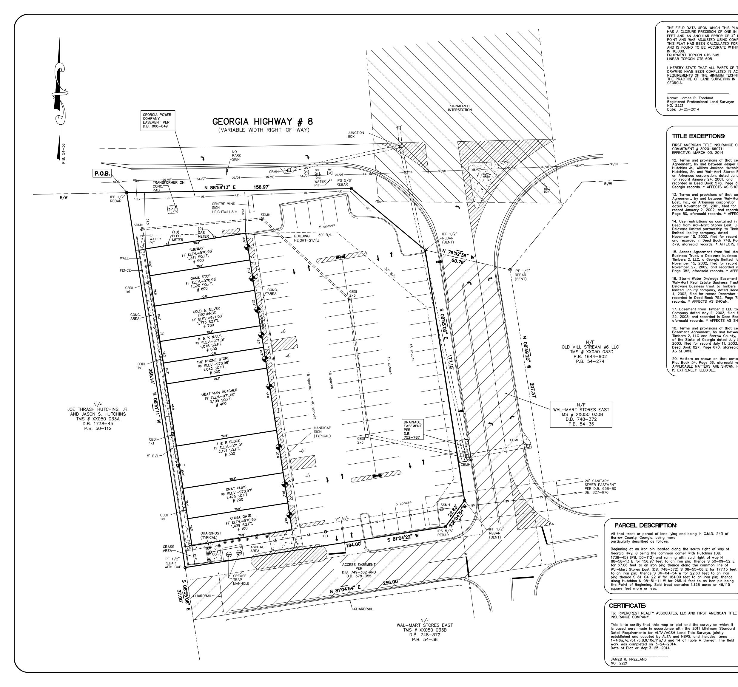
THE FIELD DATA UPON WHICH THIS PLAT IS BASED HAS A CLOSURE PRECISION OF ONE IN 10,000 FEET AND AN ANGULAR ERROR OF 4" PER ANGLE POINT AND WAS ADJUSTED USING COMPASS RULE. THIS PLAT HAS BEEN CALCULATED FOR CLOSURE AND IS FOUND TO BE ACCURATE WITHIN ONE FOOT IN 10,000.
